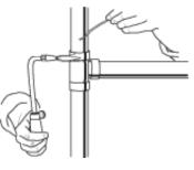
9. When the flux appears liquid and transparent on both the
