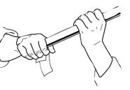
cloth may also be used with the same precautions. The cleaning should not be done with steel wool, because of the likelihood of leaving small slivers of the steel or oil in the joint.
